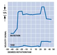
**Figure 6**—Sensor Measurement Error Versus Rotation/Yaw Angles.
