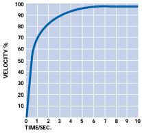
Figure 4-Sensor Flow Response.
