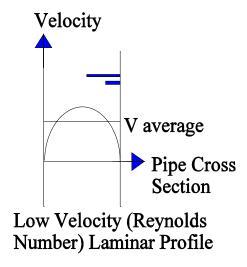
At low velocity, a laminar velocity profile develops across the pipe cross section as shown in the figure. Note that the peak velocity is about 30% higher than the velocity average (V average).
