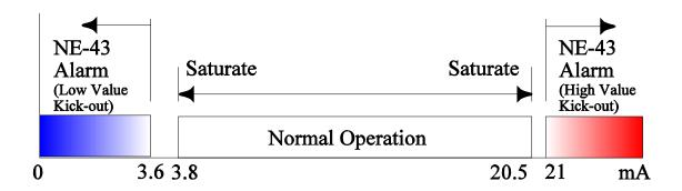
Figure 4. NE-43 Alarm signaling on the 4-20 mA outputs.
