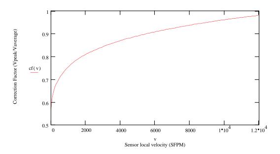
The above correction factor curve was measured from a 4" ID pipe with a ½" welded support, triple sting CD sensor. For other sized ducts, the data can be scaled by the Reynolds Number.
