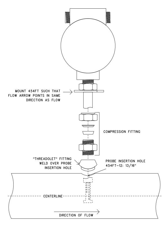
FIGURE 1 MODEL 454FT INSTALLATION WITH COMPRESSION FITTING
