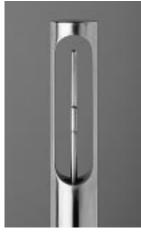
Figure 2–Fast Dual (FD) Sensor.
