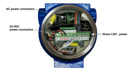
Figure 2-10. AC/DC power connection
