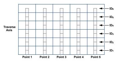
Figure B-1. Example of rectangular duct cross-section perpendicular to flow
