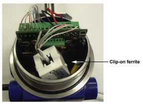
Figure 2-22. Clip-on ferrite for I/O wires
