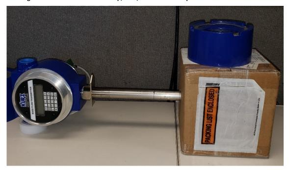
Figure C-5.Probe inside a secondary "shield" - 6x6x6 or larger box.
