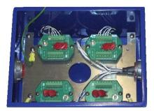
Figure 2-16. K-BAR 2000B transmitter-separate electronics example
