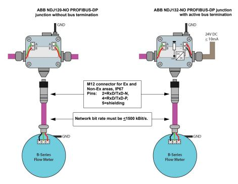
Figure 4-4. Recommended Wiring Connection with a Spur Line
