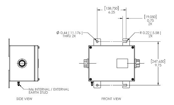
Figure 2-17. 316L Stainless Steel NEMA 4X, IP66, for Hazardous Locations
