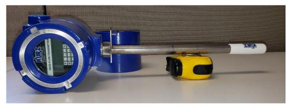
Figure C-4. Probe with flow arrow up, level, window cover in place
