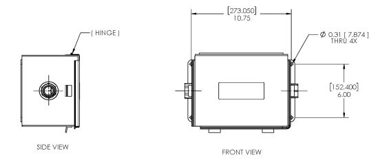
Figure 2-19. Steel NEMA 4, IP65, for General Industrial
