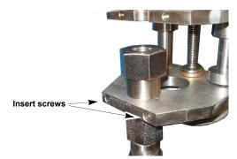
Figure D-4.Lower guide block
