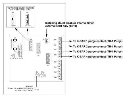
Figure 2-21. K-BAR 2000BP multipoint controller circuit board example
