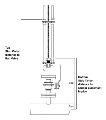
Figure D-3.Stop collar placement
