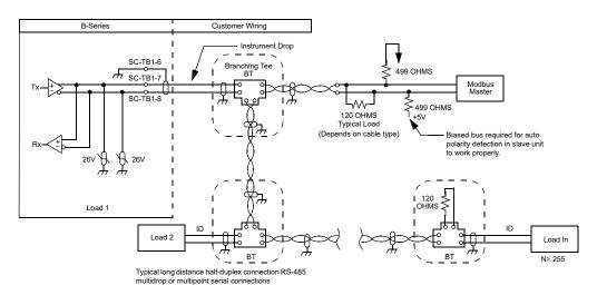
Figure 3-3. Modbus multipoint serial connections
