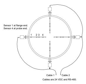
Figure 2-23. K-BAR example using Modbus communication
