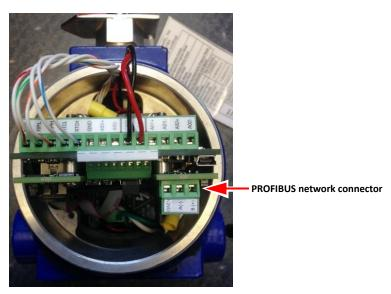
Figure 4-2. PROFIBUS Network Connector
