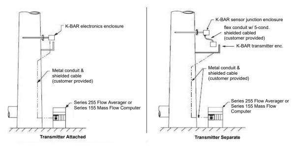
Figure 2-14. K-BAR 2000B electronics configuration examples
