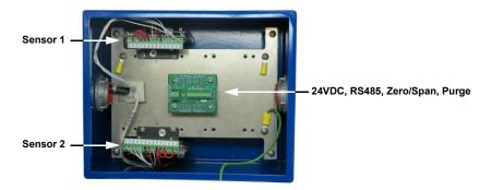
Figure 2-15. K-BAR 2000B transmitter-attached electronics example
