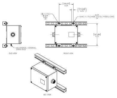
Figure 2-20. Example Enclosure Mounting using mounting rail
