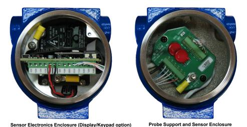
Figure 2-8. TS electronics with covers removed
