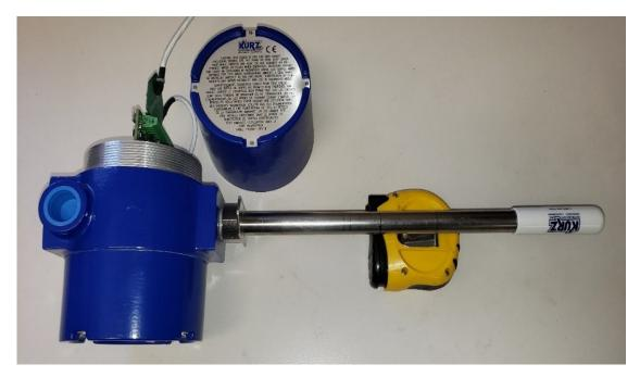
Figure C-3. Probe with flow arrow up (out of page) and window cover in place
