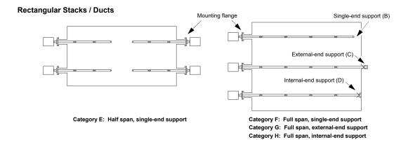
Figure 2-12. Typical K-BAR 2000B installation configurations
