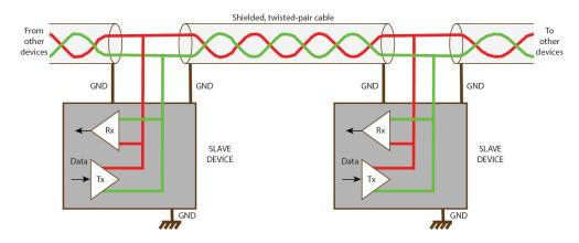
Figure 4-1. Grounding the PROFIBUS Cable
