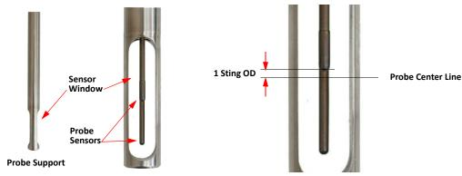
Figure 2-1. Probe support and sensors
