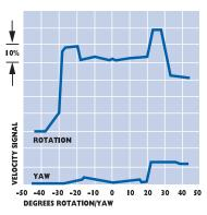
Figure 6–Sensor Measurement Error Versus Rotation/Yaw Angles.
