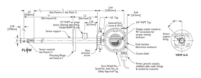
Directly Attached Dual-Chamber Electronics Enclosure Feature 1, Options A, F (Shown with Standard Display Orientation
