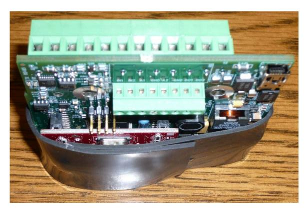
Fully loaded HART board (-14 or -17). Note the large green connector is shorter as it has one less AO.
