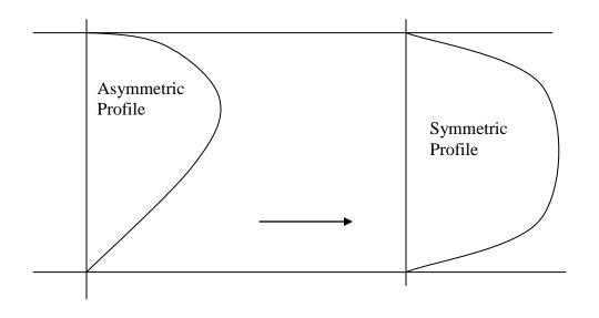
For large process piping or ducts, insertion flow elements that measure the localized or point velocity are very popular (cost effective solutions) but lack flow conditioning. For smaller process piping, an in-line meter or volumetric or mass rate meter are popular which often include some kind of flow conditioning. For that reason, the smaller meters as a group tend to have a higher installed accuracy.
