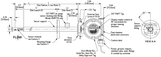
Figure AE-1. 454PFT Flow Meter. Note the ½" compressed gas port between the flange and electronics head for purge cleaning gas.
