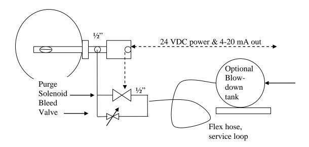
Figure AE-3. Typical system setup for 454PFT flow meter. All components available from Kurz.
