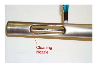
Figure AE-2. Typical purge sensor and window.
