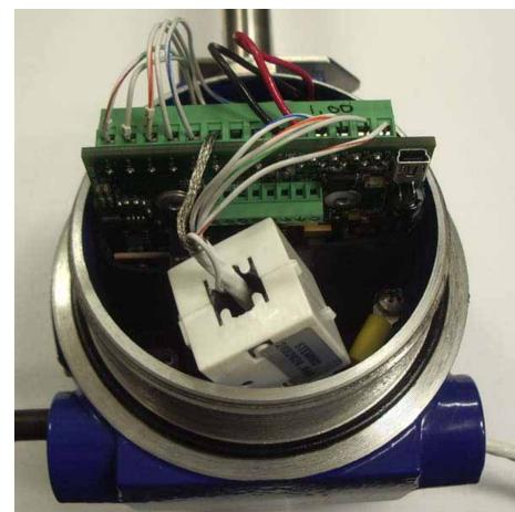
Example shows shielded 4-20 mA wiring on AO1 and AO2 with clip-on Ferrite.
