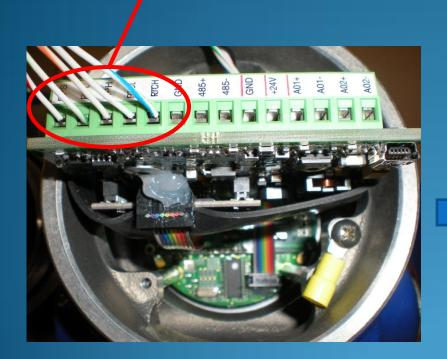
DC Power field wiring 24VDC, 21 W (18 VDC min.)
