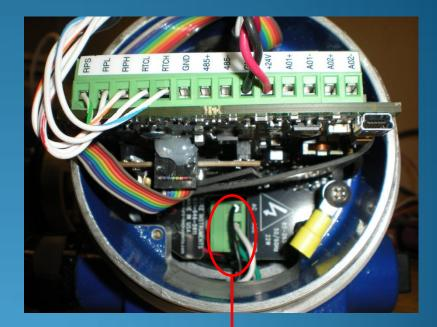
AC power field wiring installed 85-265 VAC, 50-60 Hz, 22W
