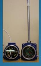
The paired enclosures must have matching sensor serial numbers as shown on the product label
