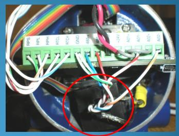
Shown here clipped around 4-20mA wiring and RS485 communication wiring
