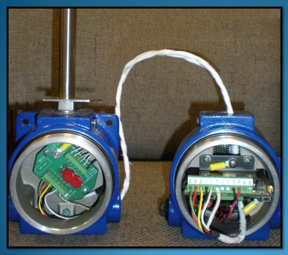
Example with short run of sensor cable attaching the electronics enclosure to the sensor junction enclosure
