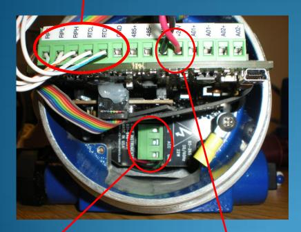
Terminal strip for customer's AC power input For AC powered meters 24VDC input is pre-wired at Kurz factory
