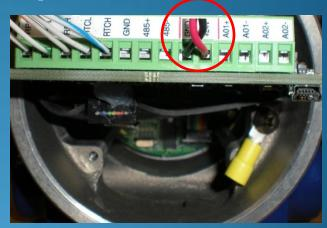
This option has no built-in power supply Customer provides 24VDC power to the meter
