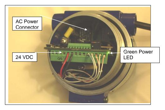
Figure AH-7. DC and AC power connection.
