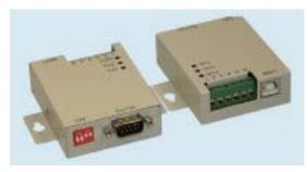
Desk computers and laptops can interface to the RS-485 devices using a USB dongle converter. We recommend the industrial version from <a href="EasySync">EasySync</a>, available from Kurz (PN 700491) or the manufacture. This device is optically isolated, screw terminal interface with metal enclosure and status LEDs, with a biased bus allowing the auto-polarity detection to work.
