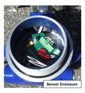
Figure AH-3. Sensor electronics enclosure and sensor J-box with covers removed
