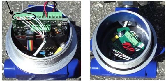
Figure A-3. Sensor electronics enclosure and sensor J-box with covers removed. Note *flow arrow* is clockwise to the sensor wiring side of the enclosure (standard orientation).
