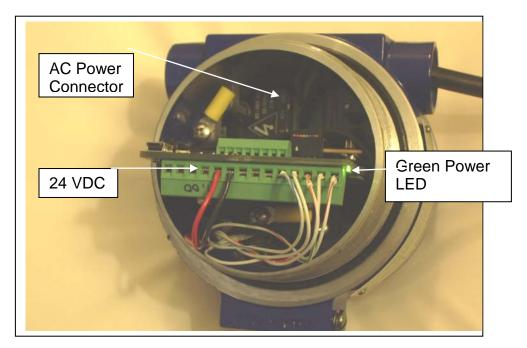
Figure A-7. DC and AC power connection.
