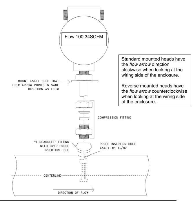
Figure A-1 Model 454FT installation with compression fitting.
