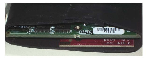
The purge version, -03 looks like the -04 fully loaded. The only way to tell the difference is to remove the board (two screws) and look under the board at the bottom as shown above. This example is the -04, fully loaded version, assembly revision B. To the right of the board version and build revision is the bar code number or board serial number. This example is A93110.
