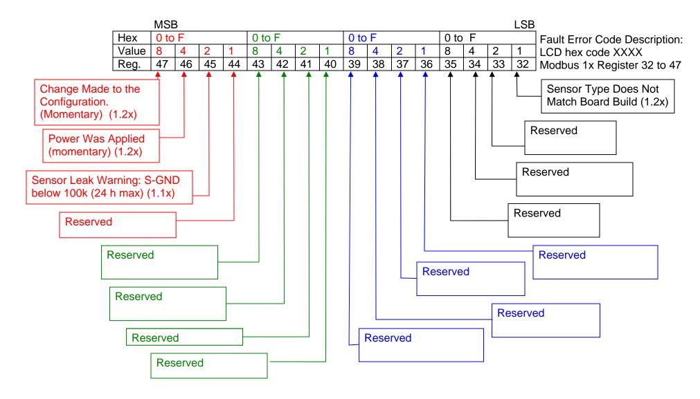
Figure E-2 Upper Word Error Code bit mapping.
