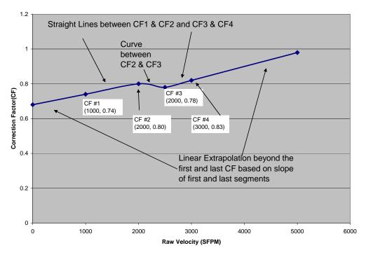
Figure AK-4. Correction Factor function with four data points.
