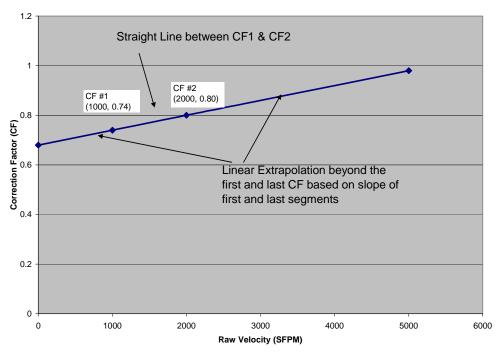
Figure AK-2. Correction Factor function with two data points.
