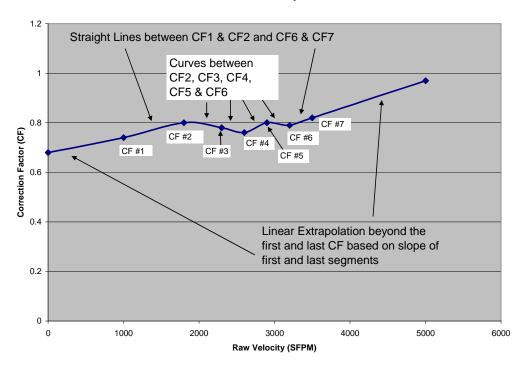
Figure AK-5. Correction Factor function with five data points.
