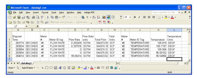
The above data were captured with HyperTerminal and saved as a .csv file. This was then opened directly by Excel then column labels were added by hand for this illustration.
