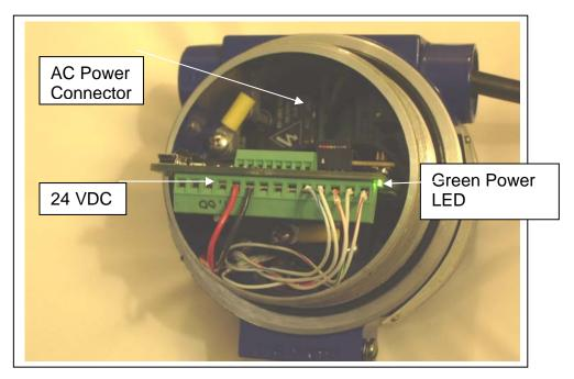
Figure AH-7. DC and AC power connection.
