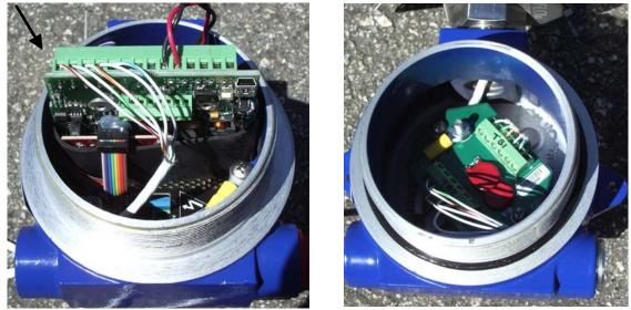
Figure AH-3. Sensor electronics enclosure and sensor J-box with covers removed
