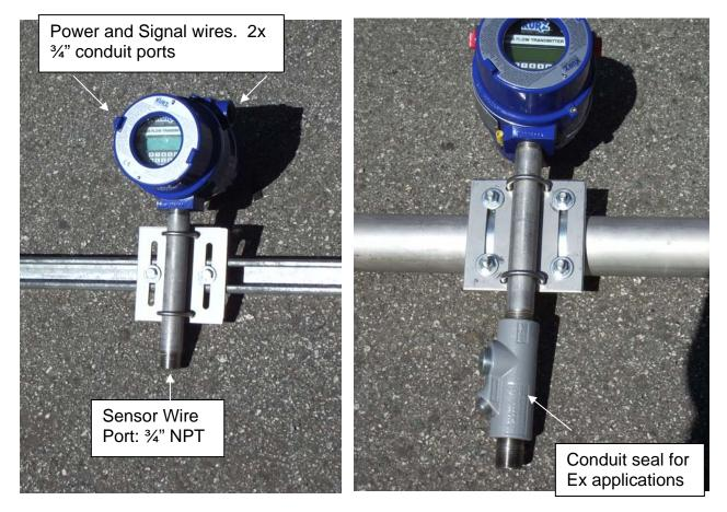
Figure AH-4. Examples of Unistrut and Pipe mounting of the TS configured electronics using the optional mounting kit, 700494-.
