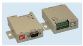
Desk computers and laptops can interface to the RS-485 devices using a USB dongle converter. We recommend the industrial version from <u>EasySync</u>, available from Kurz (PN 700491) or the manufacture. This device is optically isolated, screw terminal interface with metal enclosure and status LEDs, with a biased bus allowing the auto-polarity detection to work.
