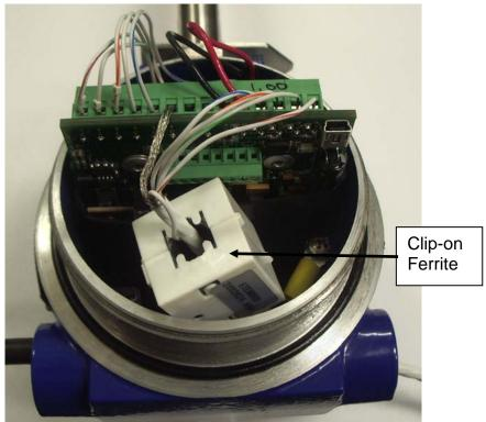
Figure AH-9 Clip-on Ferrite for I/O wires to be CE compliant without proper cable or conduit shielding.
