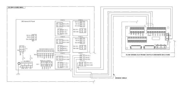
Figure 2-14. Example — Wiring from a Series 255 to a Single-Point 454FTB (Transmitter-Separate, polycarbonate)
