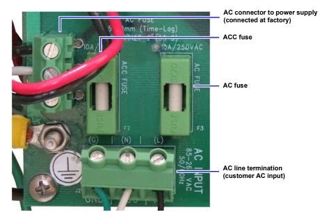
Figure 3-2. AC Power Connections
