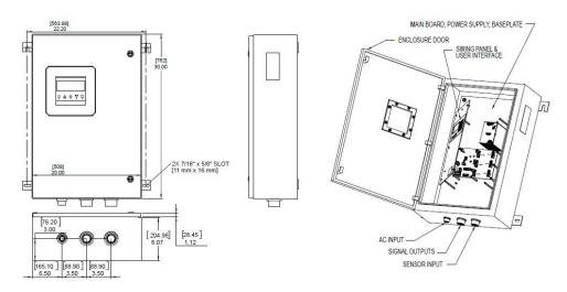
Figure 2-4. Stainless Steel Enclosure for Hazardous Locations
