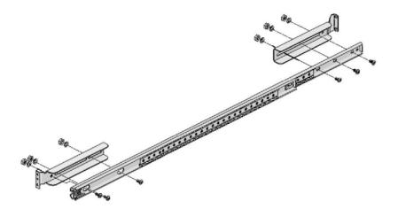
Figure 2-5. Rack Mount Slide Rails Bracket Adjustment Screws
