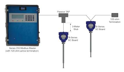
Figure 2-16. Daisy Chained Flow Meters in a Configuration using Short Stubs
