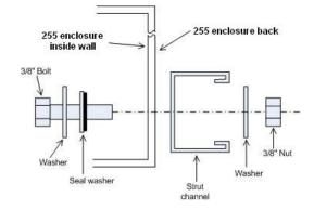
Figure 2-3. Stainless Steel Enclosure — Mounting Hardware Stack Detail
