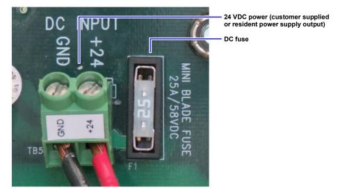
Figure 3-3. DC Power Connections
