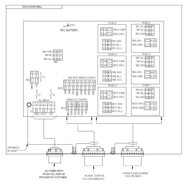
Figure 2-10. Terminal Connection Layout
