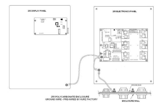
Figure 2-8. Ground Bonding for Polycarbonate Enclosures
