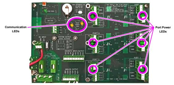
Figure 2-20. System Board LEDs
