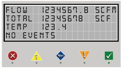
Figure 2-21. Example — Front Panel Status Indicators, System Operating Without Error
