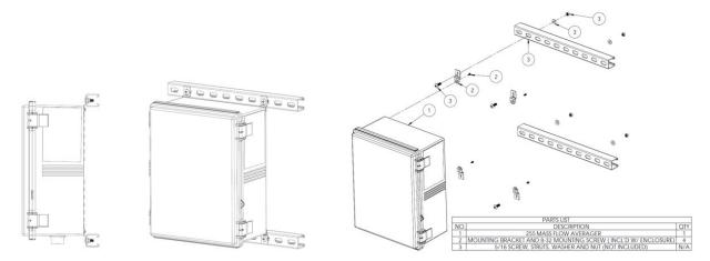
Figure 2-1. Polycarbonate Enclosure — Rail-Mounted Example
