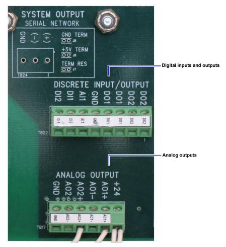
Figure 3-4. System Input and Output Communications
