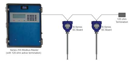
Figure 2-15. Daisy Chained Flow Meters in Recommended Configuration
