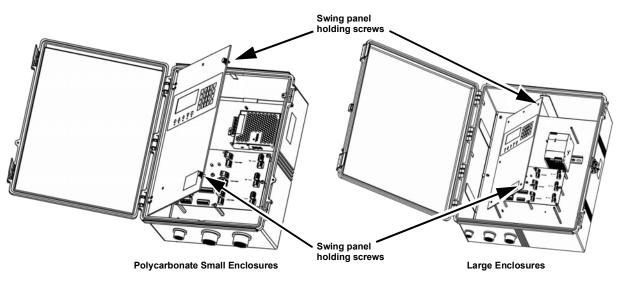
Figure 2-11. Swing Panel Holding Screws
