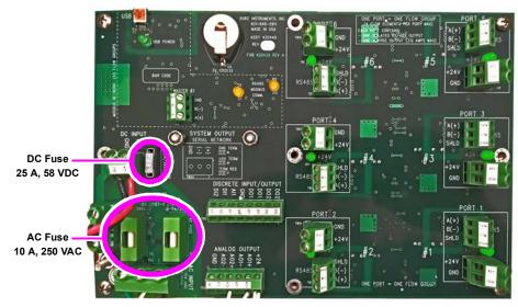
Figure 2-22. Location of System Board Fuses
