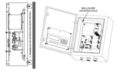
Figure 2-2. Stainless Steel Enclosure — Inside Mount Example
