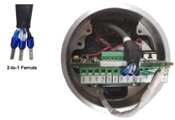
Figure 2-17. Example of 2-to-1 Ferrule used with a Single-Point Flow Meter
