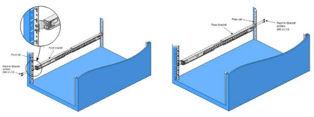
Figure 2-6. Rack Mount Slide Rails Attached to Rack Frame
